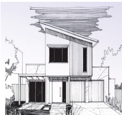
Skillion roof line
