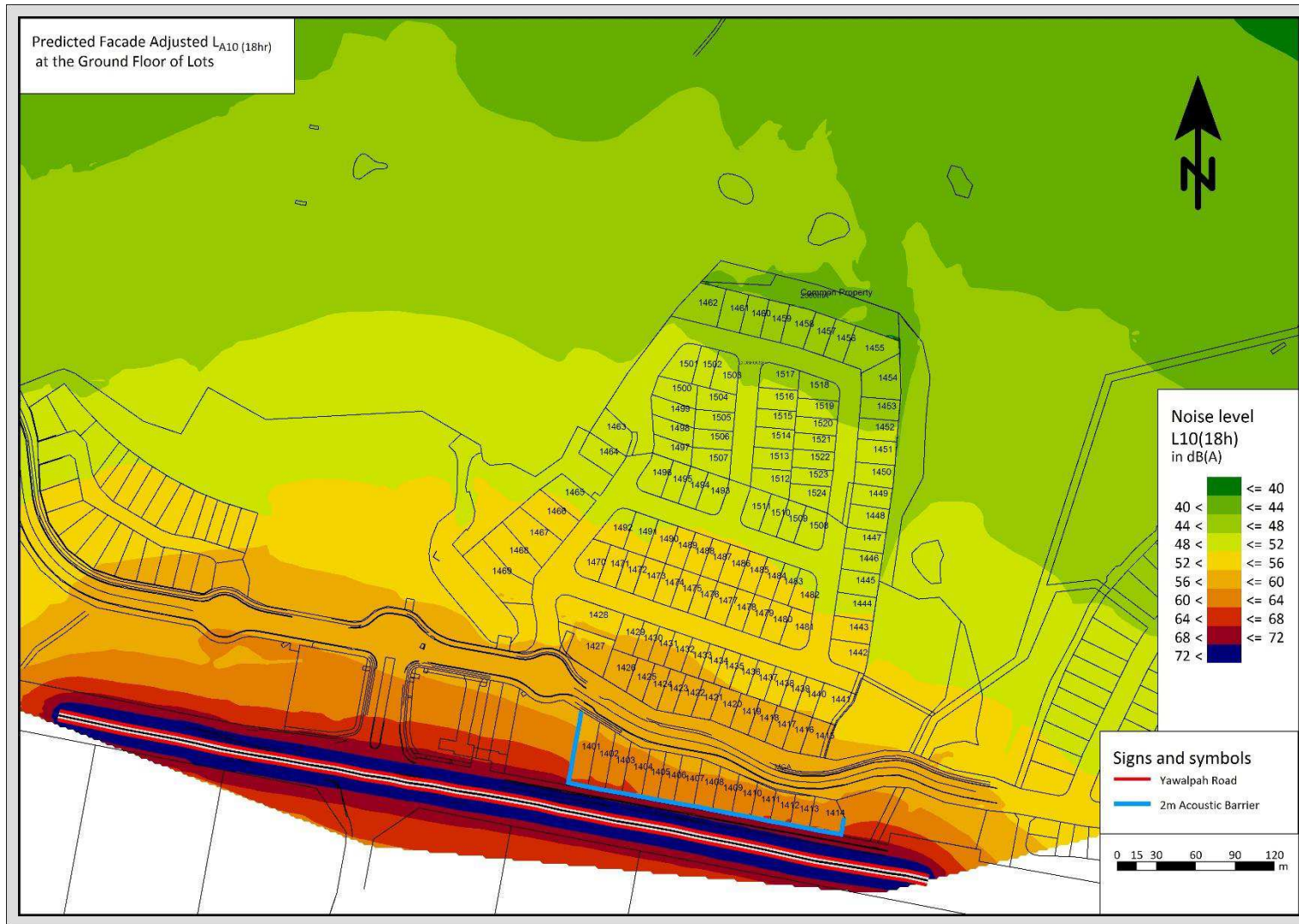
Figure E-2: Predicted Façade Adjusted LA10 (18hr) Road Traffic Noise Levels at the Ground Floor of Lots
