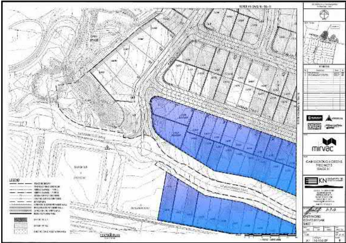
Pictures 1 & 2: Site plans showing fill areas.
