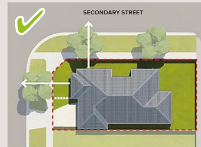
Example of compliant articulation along secondary frontage
